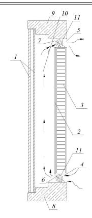
Energy-active design of the enclosure with a thermo-accumulating layer
