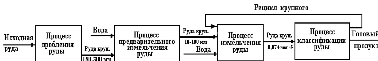
Figure 1 – The structure of the ore preparation stage
