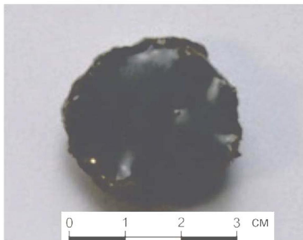
Figure 2 – Photo illustration of the product of firing clay loam (lower the horizon, the village of Ungurtas). The temperature-temporal parameters of firing stone material in a high temperature heating to 1200^{\circ}\text{C} (5', 40', 30')
