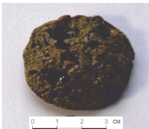
Figure 5 – Photo illustration (5) of the product of calcination of ash of a new storage (Boraldai TPP); thermal-temporal parameters of firing stone material in a high temperature heat of 1300°C (5', 30', 40')
