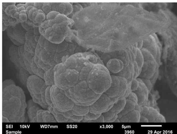
Figure 2 – A microphotograph of a gray nickel powder produced at polarization with impulse cathodic current in an ultrasonic field at a frequency of 35 kHz
