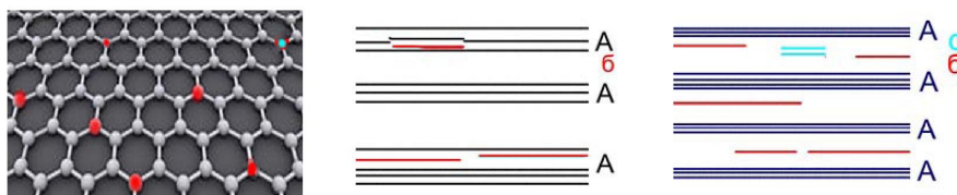
Occurrence of an impurity in layers of graphite: a – the layers forming graphite; b, c – impurities.
