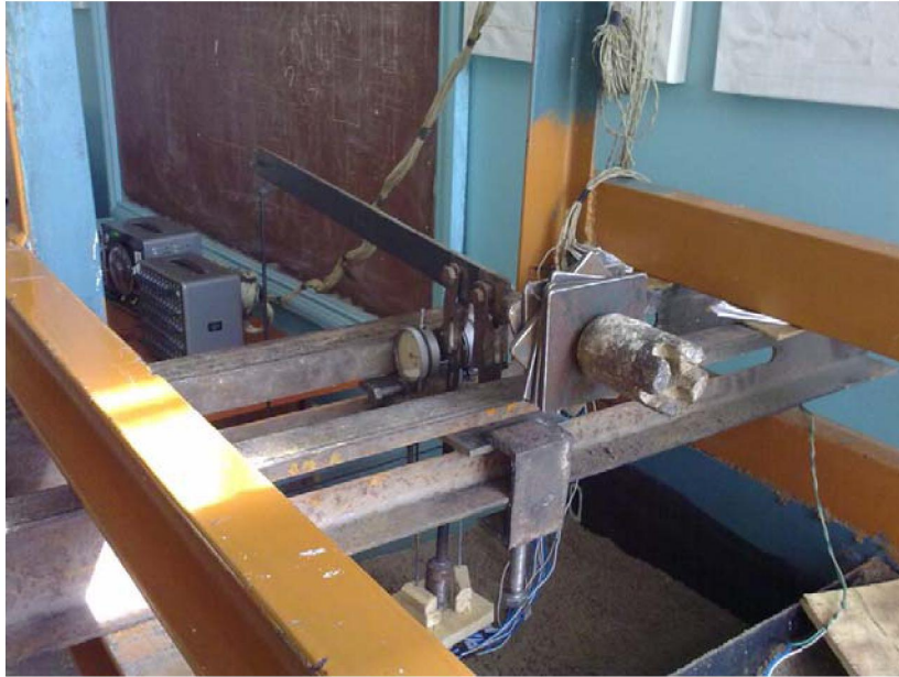
Figure 1 – General view of the static tests of model pile vertical load pressure.
