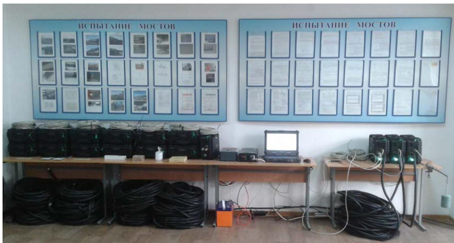
Figure 1 - Tensometric measuring and computing complex for measuring relative strains and stresses in structures
