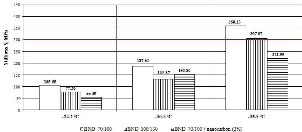
Figure 3 - Stiffness values of the bituminous binders at low temperatures t=60 s
