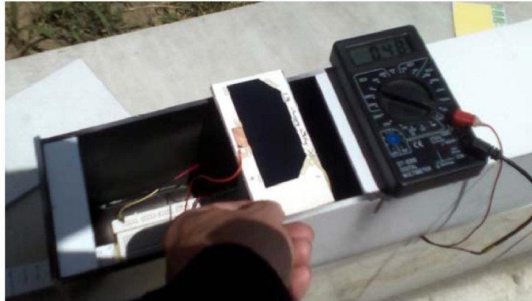
Figure 10 – Establishing the photoconversion power of gallium arsenide (GaAs)
