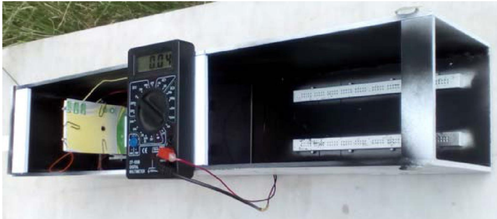
Figure 8 – Measuring the photoconversion voltage and current over the area of 0.25 cm 2
