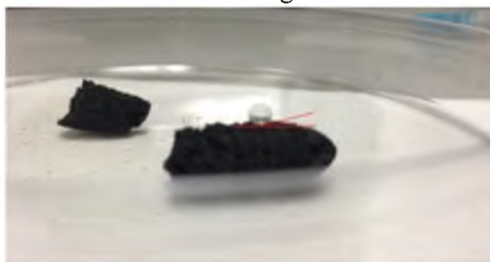
Figure 5 - The image of a water drop on the surface of synthesized MWCNT/chitosan based aerogels with indicated contact angle
