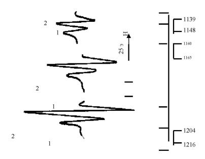
Figure 1- Change of EPR signal of oils in the section of the Kotyrtas North field, well 23. Deep: a - 1139-1148 m, b-1160-1165 m, c -1204-1216,5 m; EPR signals:1-from V<sup>4+</sup>,2-from FR
