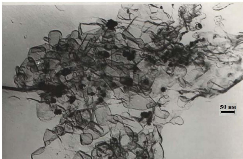
Figure 7 - Micrograph (TEM) of 1%Pd-Ag(3:1)-PAA/ZnO
