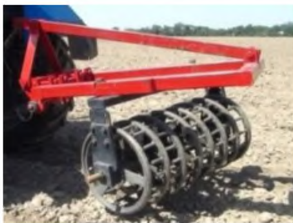
Figure 3 – Ring-bar roller on testing
