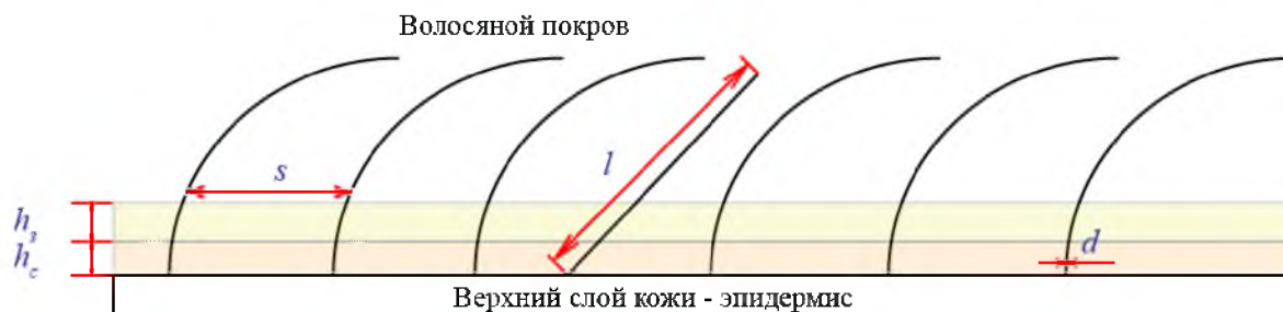
Figure 1 – Characteristics of the skin. ( s - the distance between hairs, l - hair length, d - hair diameter, h_c - thickness of natural contamination layer, h_3 - thickness of external contamination layer). Волосяной покров – hair; Верхний слой кожи – эпидермис - epidermis
