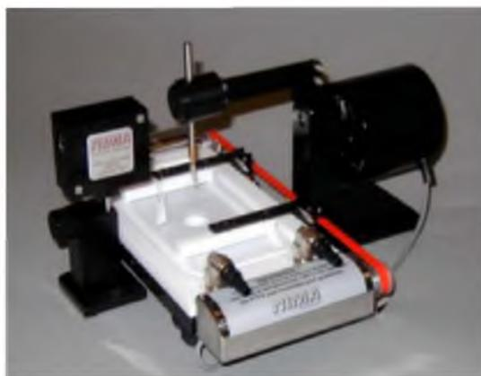
Figure 1 - A typical LB film deposition instrument (Nima CD)
