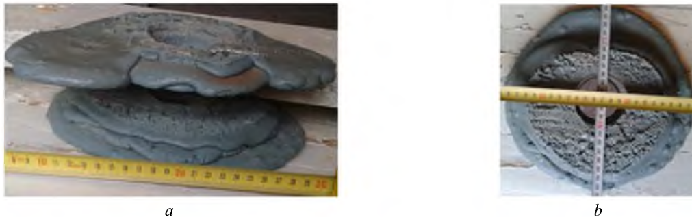
Figure 3 – Radius of TCM extent in the crack with opening of 30 mm: a – backfill stone in the level model, b - overhead view
