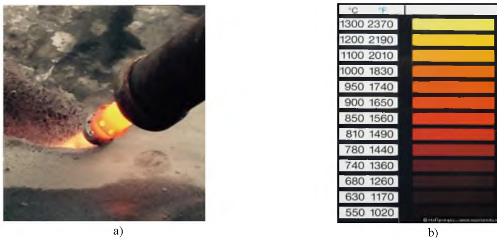
Figure 4 – The comparative analysis of heating temperature of a surface a thermal tool nozzle according to metal temperature on its color [15]: a – process of the surface treatment of thermal tool with gasdynamic nozzle; b – estimation of metal temperature nozzle on its color
