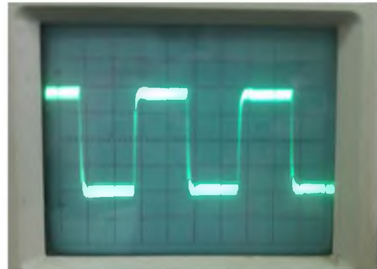
Figure 6 – Waveform of the voltage at the output of the inverter with a capacitor in the primary circuit of the transformer
