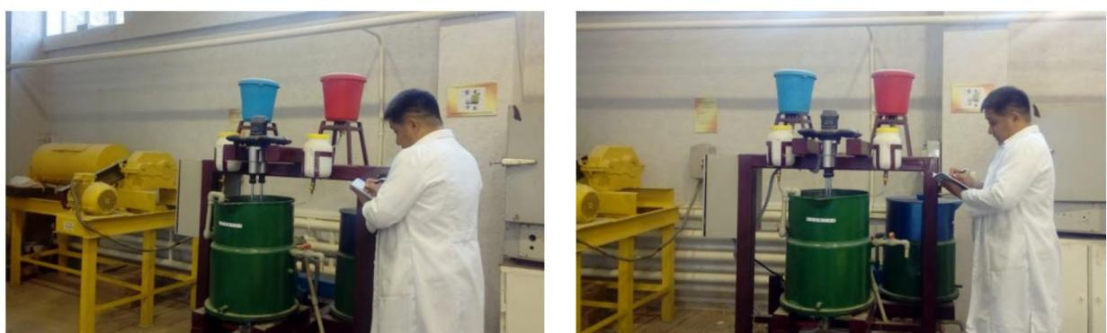
Figure 2 – Non-standard equipment for producing paraffin compositions
