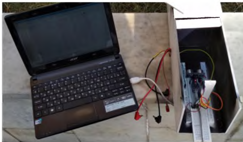
Figure 5 – The digital system for measuring the qualitative characteristics of holographic concentrator samples
