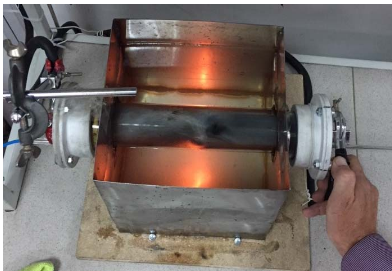
Figure 1 - Installation for producing CNTs by electrophysical method
