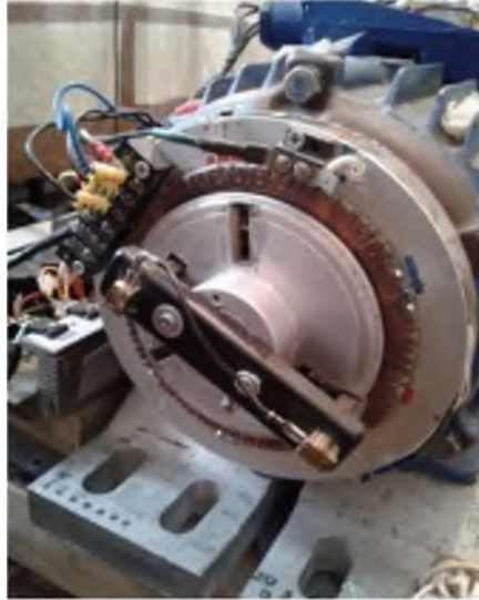
Figure 5 – Photo of manifold with contactors
