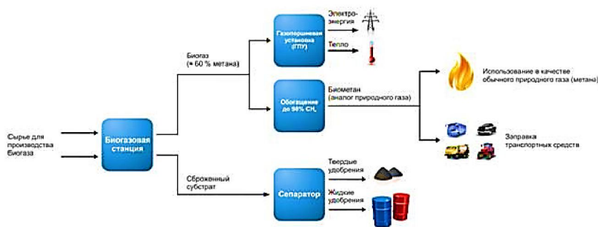
Figure 2 – System of receiving and combustion of biogas
