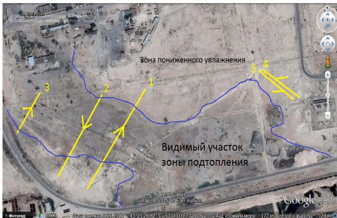
Picture 4 – Scheme location GPR and numbering geophysical profiles on the area under flooding in the region GPP
