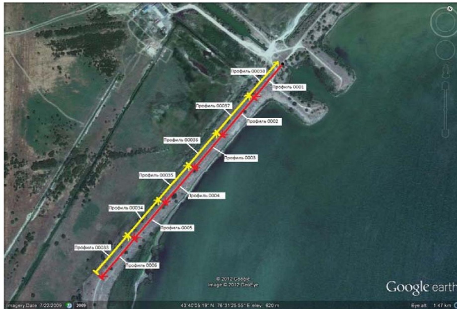
Picture 1 – Schematic layout of geophysical profiles on the 1st dam wastewater reservoir «Sorbulak»
