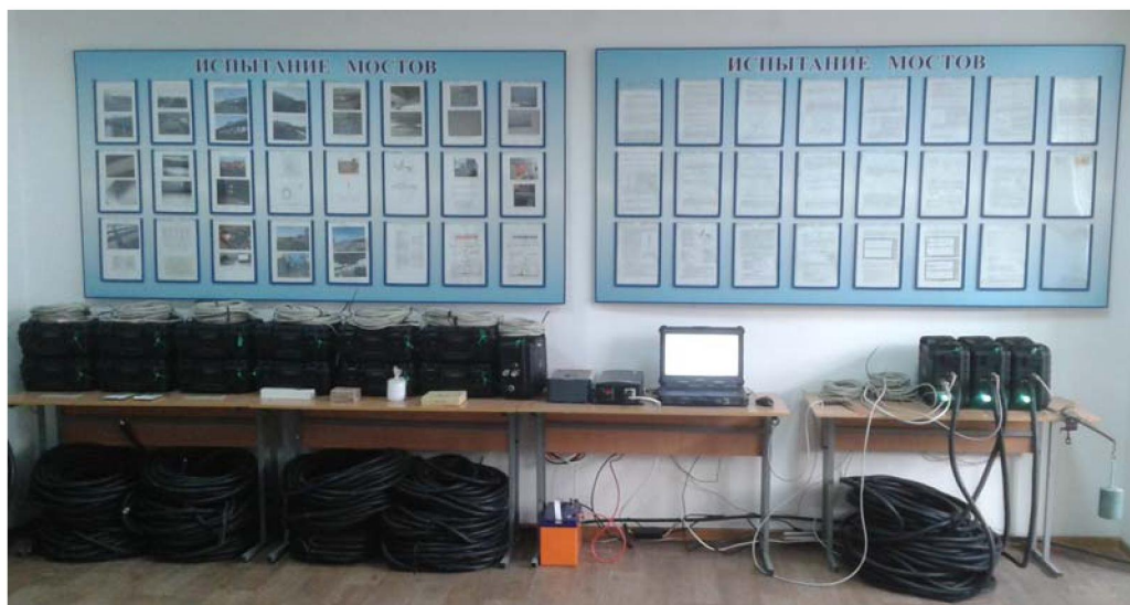
Figure 1 – Tensometric measuring and computing complex for measuring relative strains and stresses in structures
