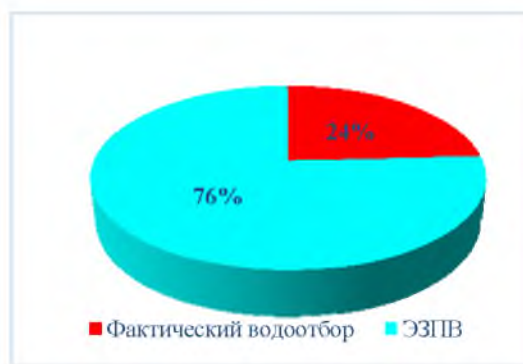
Figure 4 – Diagram of the use of the operational groundwater resources in the state balance in the Almaty metropolitan area
