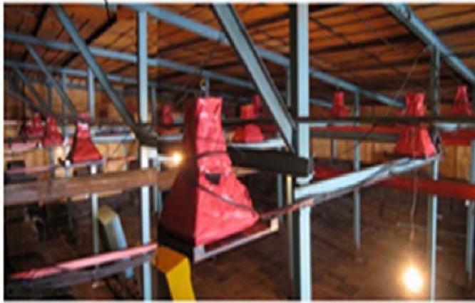
Figure 1 – Scintillation detectors installed in the launch building
